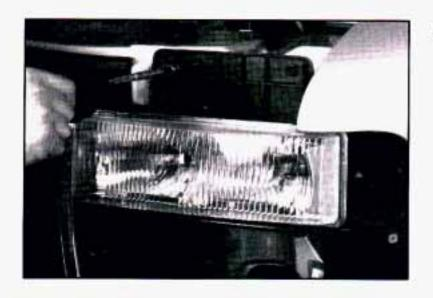
Remove the remaining three screws; the first one from the corner reflector pocket and the two remaining from the composite assembly.
